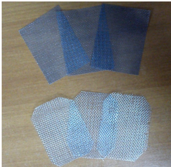
Fig. 1. Plastic meshes: a polymer fiber (fiberglass) coated with PVC (top) and a metal mesh (aluminum) (bottom)
