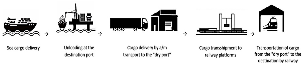
Fig. 1. The scheme of cargo transportation through the “dry” container terminal
