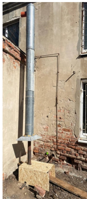
Fig. 3. Experimental setup with a casing installed to create a slit channel
