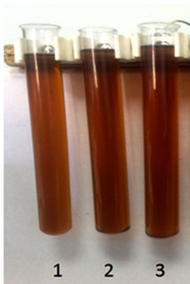
Fig. 2. The samples of the lubricants for tribological testing: 1 – an oil M-16G2CS; 2 – a lubricant composition “oil M-16G2CS + 1.0% of the additive”; 3 – a lubricant composition “oil M-16G2CS + 2.0% of the additive”
