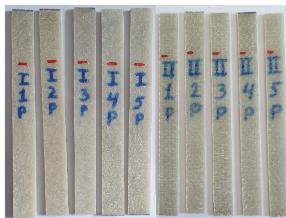
Fig. 7. Samples of two different reinforcement schemes from the edge treatment with polyester resin to the tensile test
