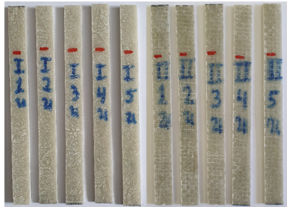
Fig. 3. Samples of two different reinforcement schemes from the edge treatment with polyester resin to the three-point bending test
