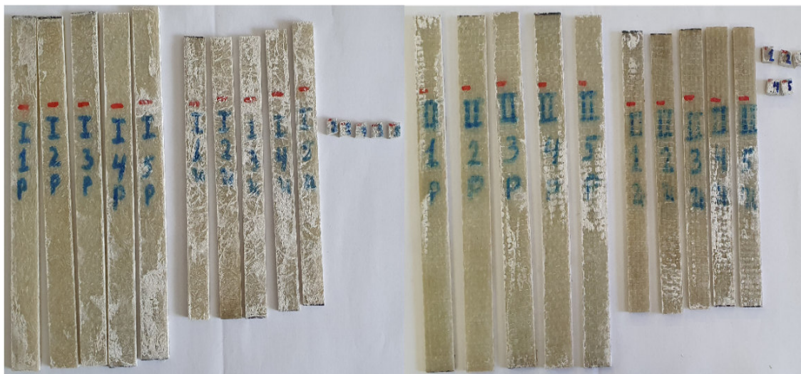
Fig. 1. Samples from the PCM of two reinforcement schemes with treated edges with polyester resin after soaking in water
