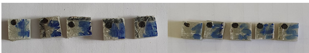
Fig. 10. Samples of two different reinforcement schemes without edge treatment with polyester resin for compression testing
