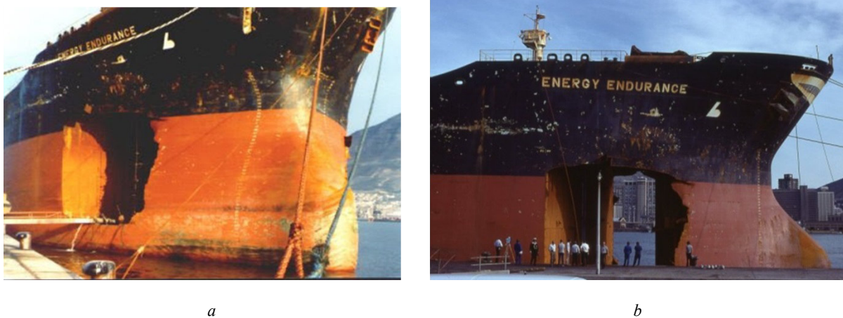
Fig. 2. Damaged bow of the Energy Endurance tanker [6]: a – front view; b – side view
