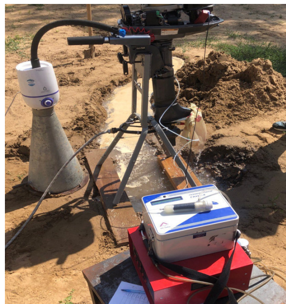
Fig. 4. GANK-4 gas analyzer with a probe inserted into the deadwood hole of the OM and a tachometer sensor installed during testing in the open air
