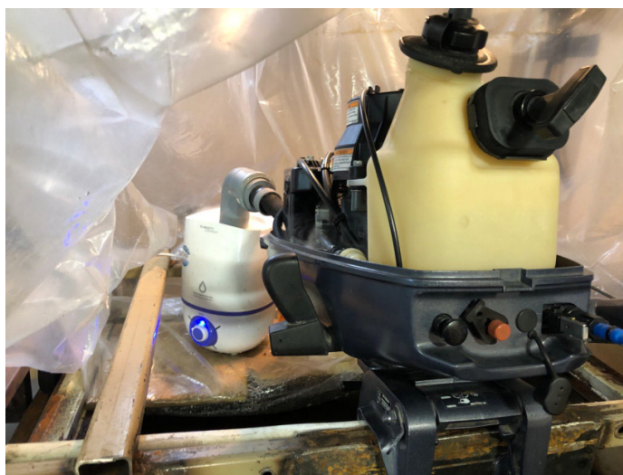
Fig. 3. Outboard boat motor Yamaha F4BMHS 4 hp was installed in a small experimental pool with a water supply option from an external source
