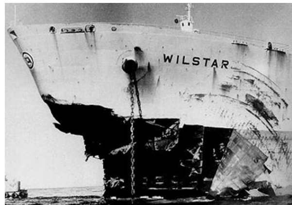
Fig. 2. Damage to the bow of a large vessel caused by rogue waves
