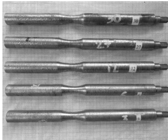
Fig. 4. Specimens for fatigue testing
