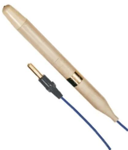
Fig. 2. Second-class reference electrode with ShP 4-2 plug manufactured by GOMEL (general view)
