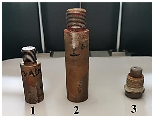
Fig. 1. General view of the steel protectors under study: 1 – factory-made steel protector (No. 1); 2 – self-made steel protector (No. 2); 3 – self-made steel protector (No. 3)
