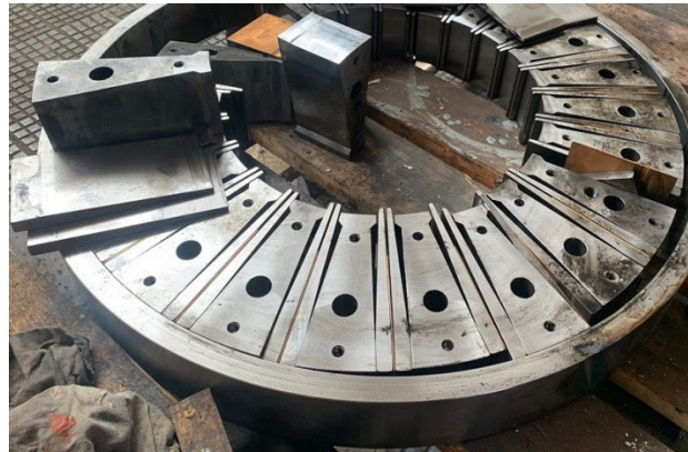
Fig. 5. Reverse engineering of the Geislinger D60/14/2 damper
