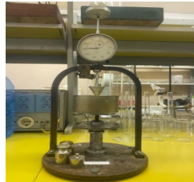
Fig. 7. External view of the penetrometer with the sample before immersion of the cone
