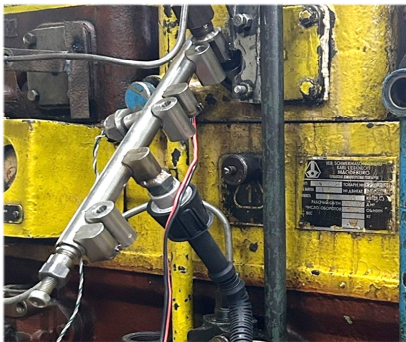
Fig. 2. Installed nozzle for supplying additional components to the 1Ч17.5/24 diesel cylinder
