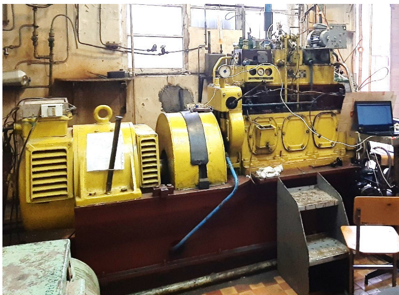
Fig. 1. General view of the test bench for supplying additional components to the 1Ч17.5/24 diesel cylinder
