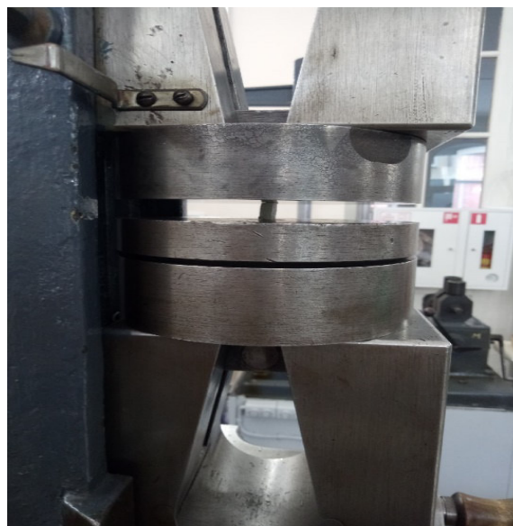
Fig. 11. Compression testing PCM samples on the R-5 machine
