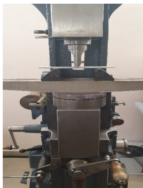
Fig. 3. Testing PCM samples on the R-5 machine for a three-point bend
