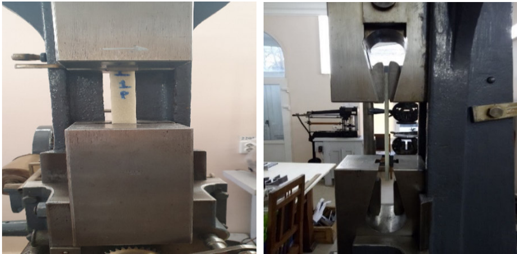
Fig. 7. Tensile testing PCM samples on the R-5 machine
